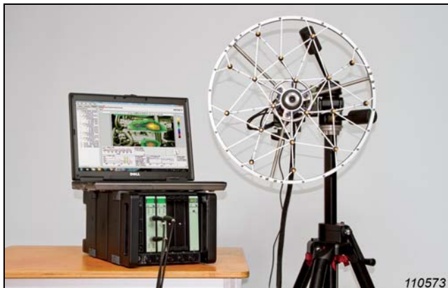
Fig. 19 Front Panel UA-2112 being used in an array application
