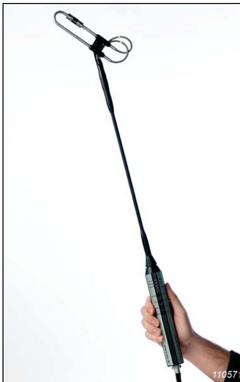
Fig. 9 Left: Sound Intensity Probe Kit Type 3599 Right: Pin-out for the LEMO (7-pin) connector
